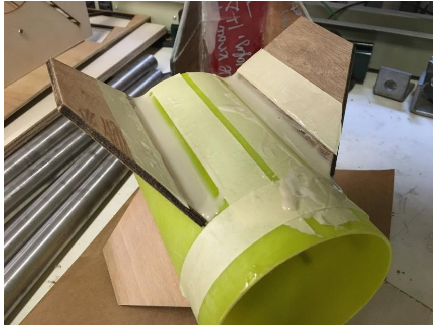
Figure 2-3: Practice Fillets on a Spare Piece of Airframe Tube
