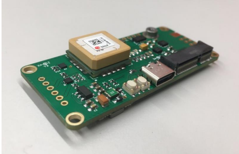
Figure 3-12: Assembled Flight Computer Circuit Board
