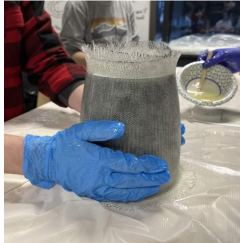
Fig. 25 Fiberglass lay-up of Tailcone
