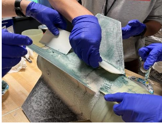
Fig. 23 Applying Bondo Glass to Fin Can
