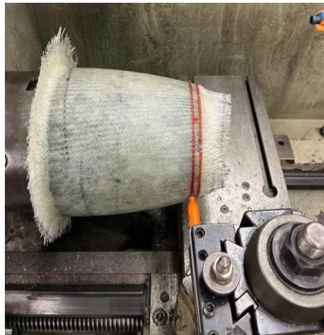
Fig. 26 Marking Fiberglass Tailcone for Dremeling
