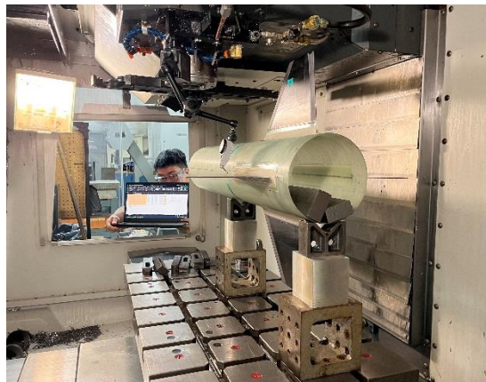
Fig. 21 Utilizing Dial Indicator in a CNC Mill to Measure Positional Data of each Fin
