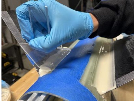
Fig. 20 Building up Rocketpoxy Fillet along Fin Root
