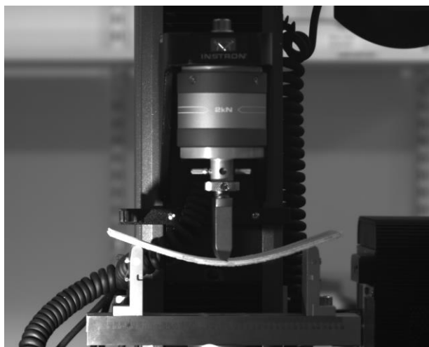
Fig. 13 Three-point Bending Test of Sandwich Composite Coupon
